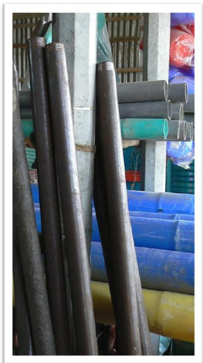
18 Additional Extension Piping for Tube Wells
